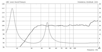
1) Drive voltage of 2.2Vrms chosen to provide 1W to the loudspeaker at 40Hz. Zmin=3.2Q, Znom=5.9Q from 32Hz to 150Hz. 2) 1012W @ 90Vrms / 8Q AES2-2013 2hr test. 2400W @ 90Vrms / Zmin=3.3Q AES2-1984(r2003) 2hr test
